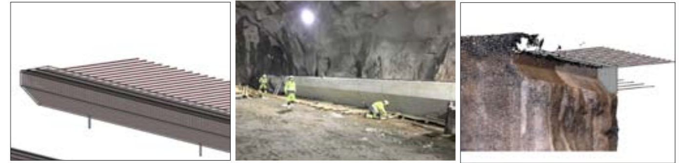
Above: Figure 8. Design basis, execution and control of geometry for concrete overhead gantry crane girder. Right: Figure 9. Example of model viewpoints.
